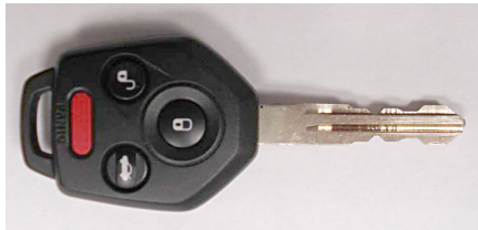
2009 Legacy & Outback and 2009-2013 Tribeca side cut key w/ immobilizer and keyless entry
