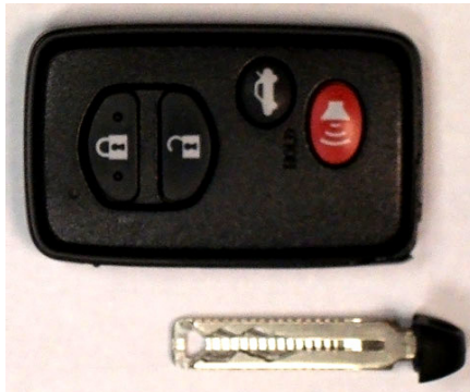
2013 BRZ keyless access with push-button start system access key with inside cut mechanical key, immobilizer, and keyless entry
